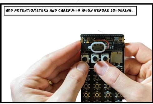
SOLDER THE POTENTIOMETERS FROM THE BACK - ALL THREE POINTS AND THE TWO WINGS AT THE BOTTOM.
